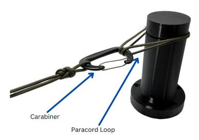
On the up-range side, feed the paracord through the tensioner system, following the diagram provided. This system provides mechanical advantage and allows for high tension to be applied to the cord. If the cord spans a short distance, the locking cam may provide sufficient tension on its own.
