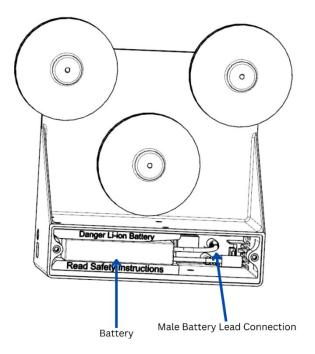
Once the battery is properly connected, reinstall the battery cover. Ensure the cover is fastened securely to prevent any potential damage or disruption to the battery during operation.  Install the antenna to the target carriage circuit board through the provided hole.
